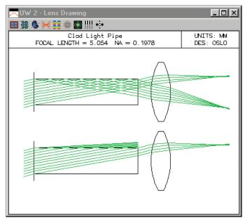
All of the usual ray trace commands are available for systems employing light pipes. However, for single ray tracing, only the ray data for the entrance and exit faces is displayed, and much of the other ray trace data (e.g., ray-intercept curves) is essentially meaningless because of the variable number of reflections in the light pipe.
