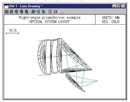
The prism will have an aperture of 10 (note that apertures in OSLO are specified by their radii, not diameters), and will be located 1 mm to the right of the last lens surface.
